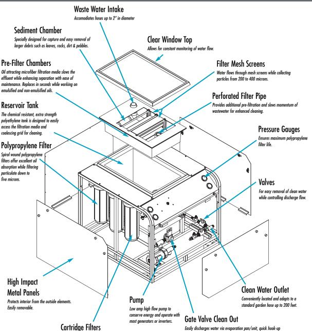
Designed for filter changes in less than 5 minutes. 100% polypropylene filter housing provides leak-proof double seals providing resistance to chemical fatigue and ultraviolet exposure. Easily discharges water via evaporation pan/unit, quick hook-up to vacuum & pump to a drum, or biological remediation system.
